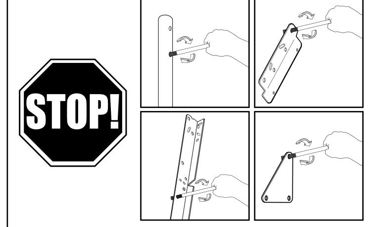
To ensure optimal playability of backboard system, a close tolerance fit between the elevator components and hardware is required. Test fit large bolts into large holes of elevator tubes, backboard brackets and triangle plates. Carefully rock them in a circular motion to ream out any excess paint from holes if necessary.
